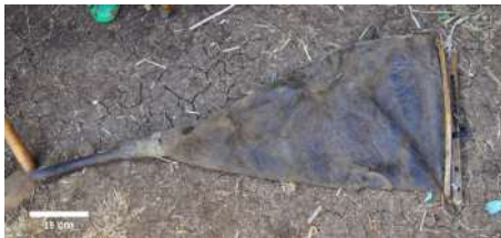
FIGURE 11 Bellows used for blacksmithing, Amba G w alit (B. Kribus/V. Krebs)
