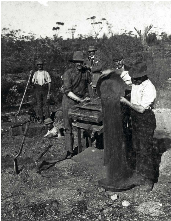
Figure 5. Dry blowing at Coolgardie using two gold pans. A breeze blowing from the back to the front deflects light material to miss the bottom dish, whereas dense particles including gold fall vertically into it. Note the shaker and screen in the background to remove largest fragments and achieve first-pass concentration before dry blowing by pans. Used with permission from the State Library of Western Australia (Call No: 3542B/350).
