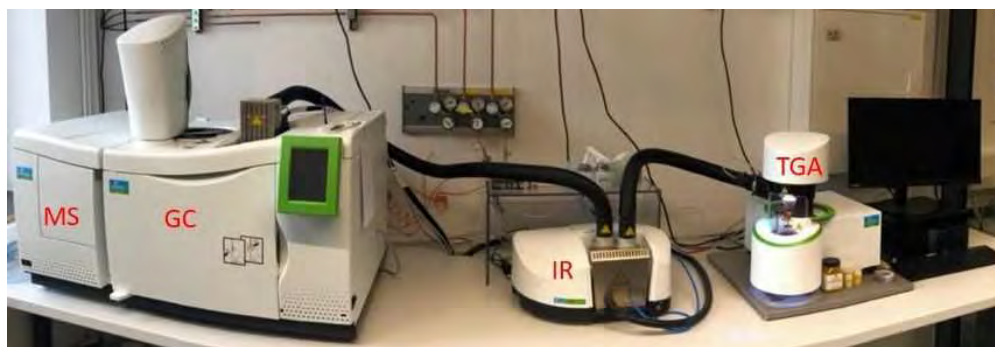
Abbildung 1: PerkinElmer-Kopplung TGA 8000- Spectrum Two IR-Clarus680/SQ8T GC/MS.
