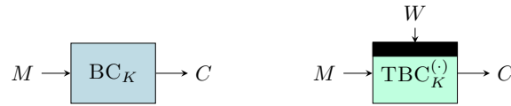
Figure 16: Block-cipher (left) and tweakable block-cipher (right). For tweakable block-ciphers, the black bar indicates that the incoming arrow ( W ) is the tweak.
